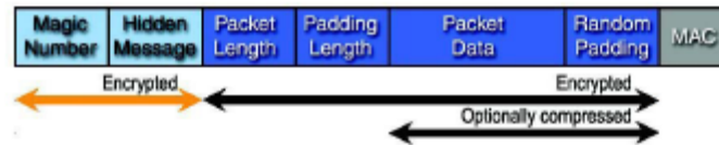
Figure 7: Adding an encrypted portion with a hidden message to a regular SSH packet.
