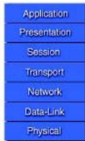
Figure 4: The OSI Idealized Network Model Layers.
